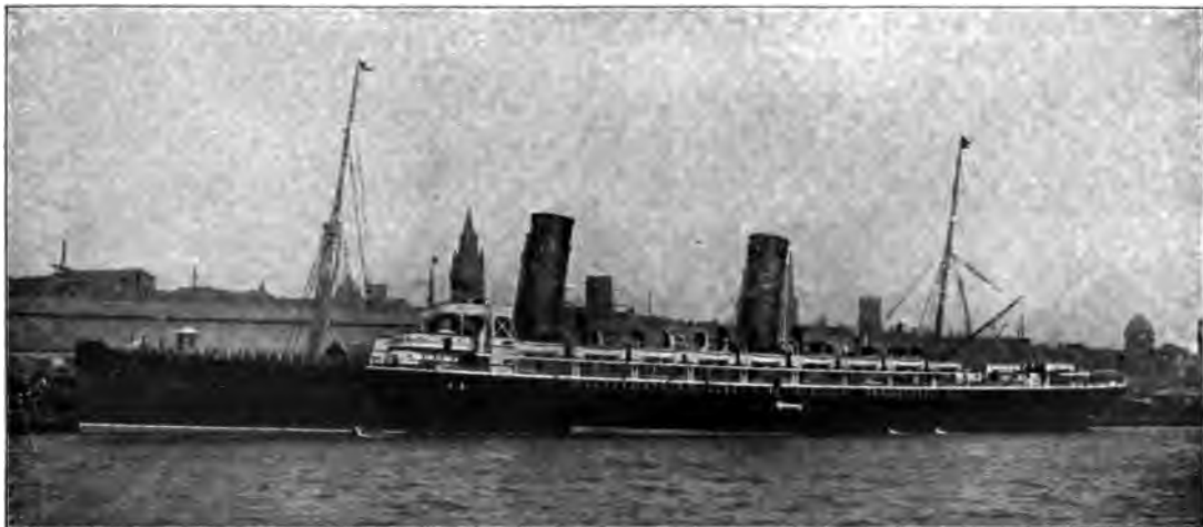
THE CAMPANIA, A PASSENGER GREYHOUND OF THE ATLANTIC. (Length, 625 feet; breadth, 65 feet; displacement, 19,000 tons; speed, 22 knots, or 25 statute miles, an hour; capacity, about 2,200 passengers.)
